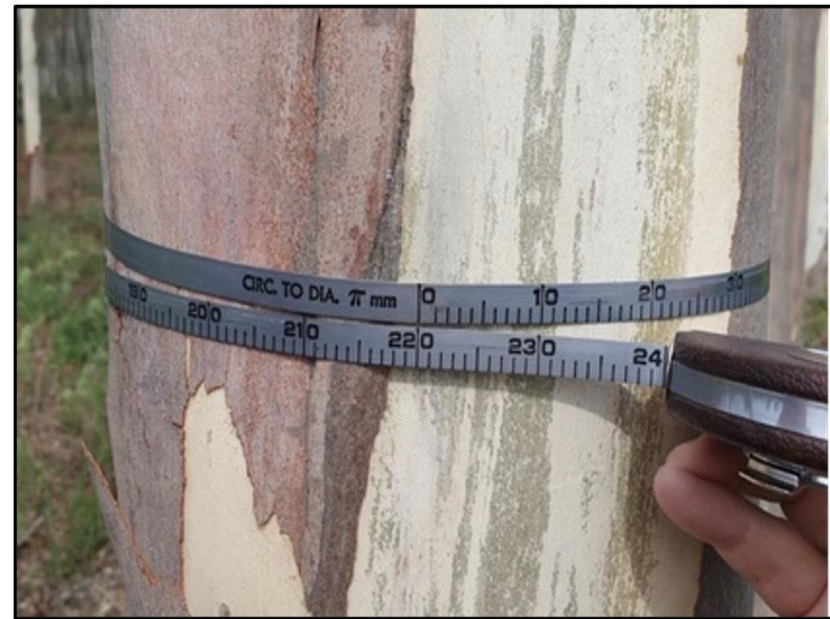
Figure 10. The diameter at breast height of a three-year-old Eucalyptus urograndis tree from the plantation in figure 7 is 22 cm (8.7 inches). Photo credit: Robert Davis (World Bank 2019).
