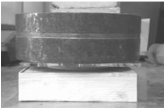
Figure 90. Water absorption test with a weight to seal the system
