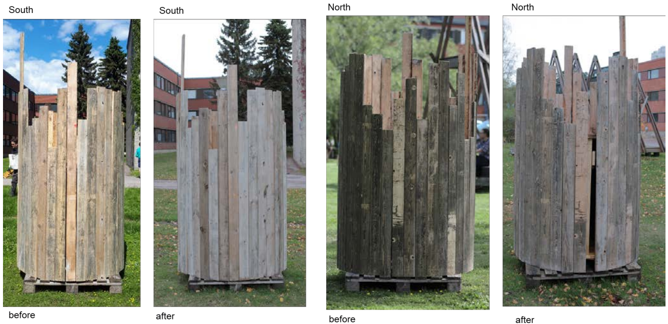
Figure 14. Comparisons of the south and north view of the full scale demonstrator at Aalto University, Otaniemi Campus, Espoo, 60°11'15.7"N 24°49'55.4"E - before and after 4 months of exposure to natural environment June to October 2022.
