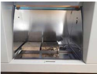
Figure 9. Suntest CPS+ device - suntest with two formwork wood samples
