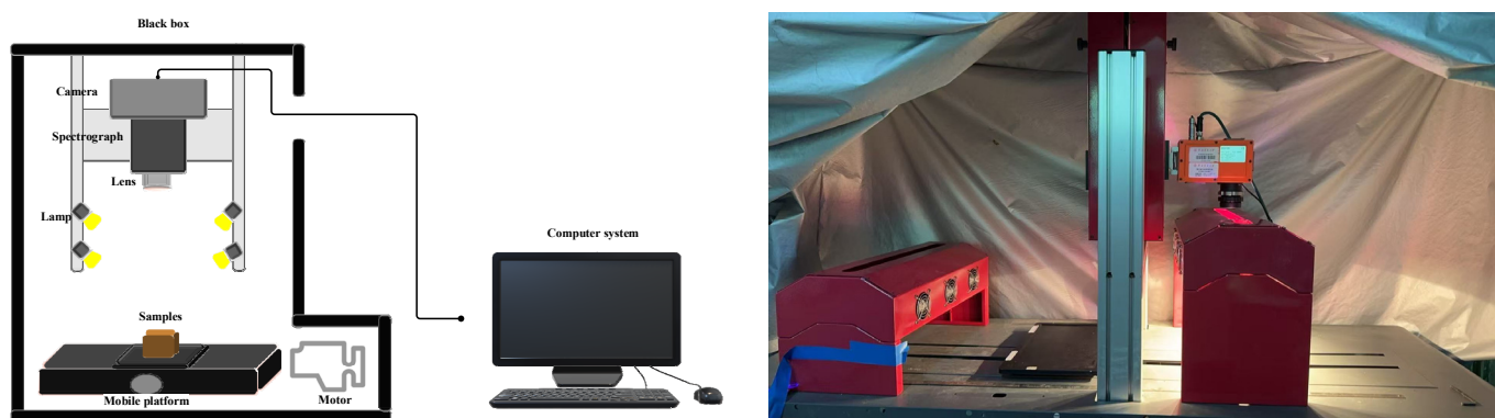
Figure 2. Diagram of VNIR and SWIR Hyperspectral Imaging Systems (VNIR: 400–1000 nm, SWIR: 900–1700 nm).
