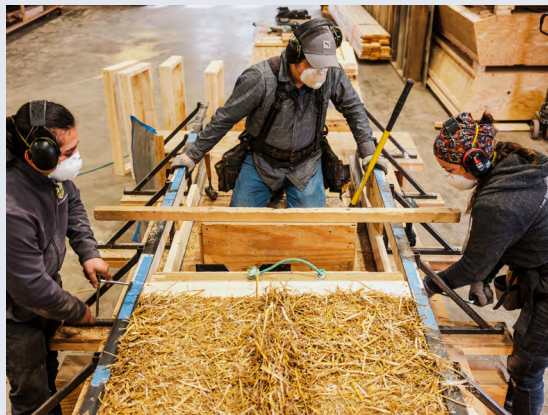
Prefabrication of structural insulated straw panels. Courtesy of New Frameworks.
