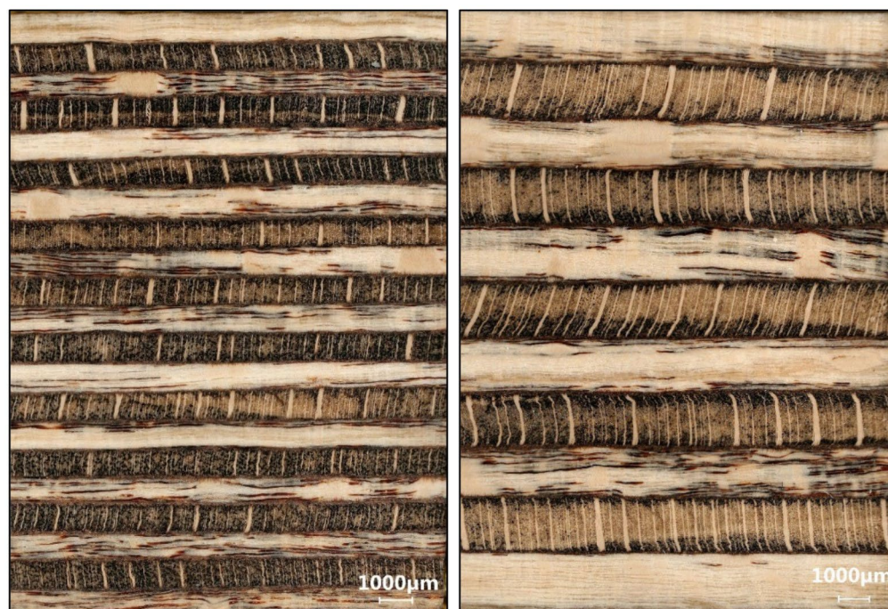
Figure 5. Microscopy of the plywood cross-section of 1 mm (left) and 2 mm veneer layers (right).
