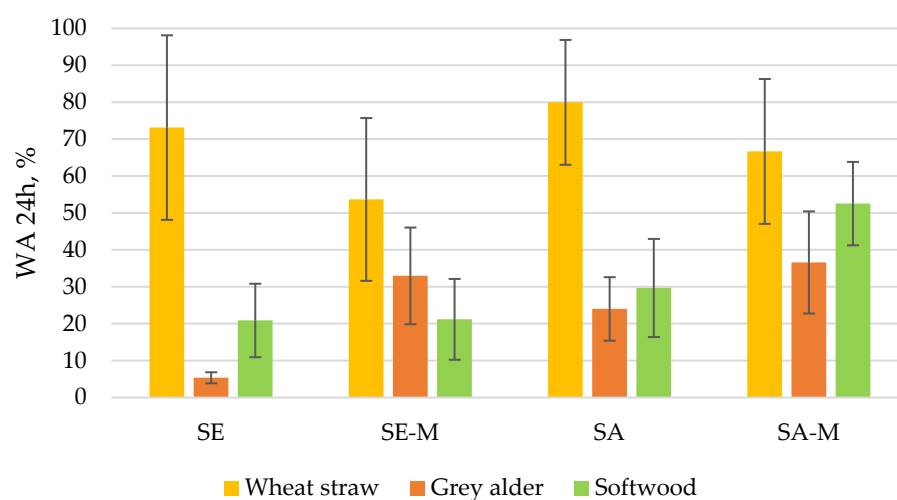
Figure 3. Water absorption of particleboards depending on raw material and board type.
