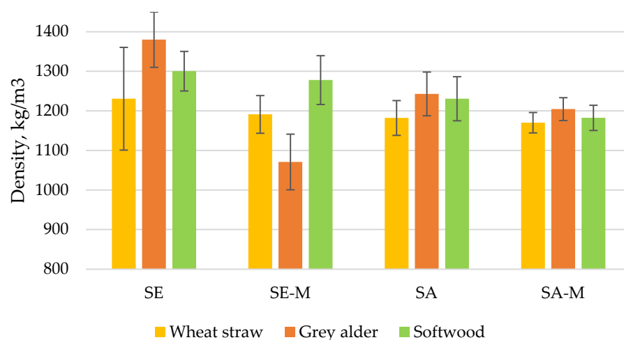
Figure 2. Density of particleboards depends on raw material and board type.
