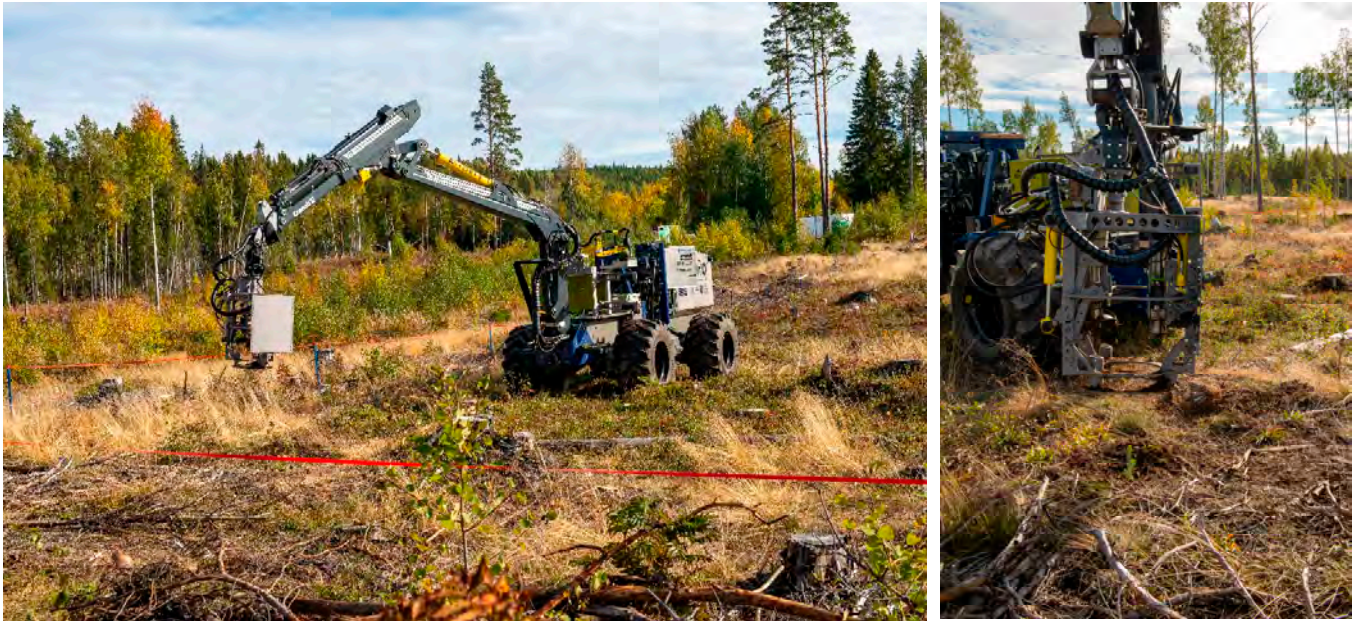
Figure 9. Autonomous site preparation and planting demonstrated for the first time in September 2022 at a forest regeneration area outside Bräcke, Sweden. (Left) The autonomous vehicle platform with the crane steering toward the self-selected planting spot. (Right) An autonomously planted seedling with the light site preparation and planting device, developed by Bräcke Forest.
